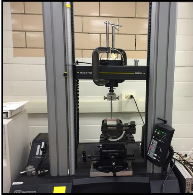
Figure 7: Specimen in place for the three-point bending flexural strength test (Instron® Model 5565 Universal Testing Machine)
